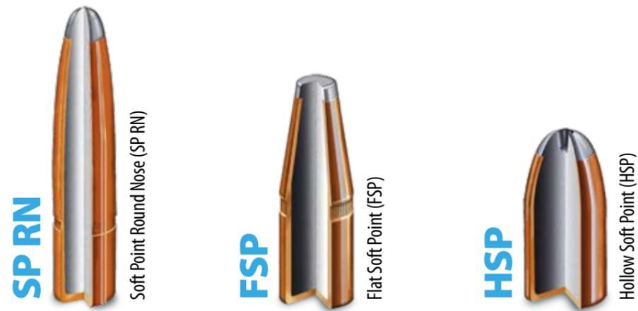
**FSP bullets** have a flat lead nose with increased diameter. These bullets are suitable for use in carbines with tubular magazines as they reduce the possibility of primer ignition in the cartridge placed in front due to recoil when firing. They expand reliably and penetrate deeply on light to medium game. HSP bullets have a cavity in the nose which causes expansion and helps mushrooming during penetration.
